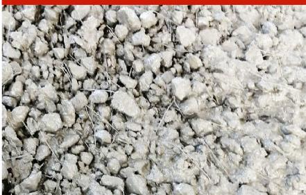
**BUNDREX 80/60CH** steel fibers are high quality structural steel fibers designed for reinforcement in Slab On Grade. They are used successfully to replace the electro welded mesh in the reinforcement of industrial floors with an excellent performance proven with laboratory tests according to EN14651 and ASTM1609 standards.
