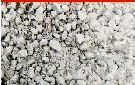
**BUNDREX 66/35CH** steel fibers are high quality structural steel fibers designed for reinforcement in shotcrete spraying. They are used successfully to replace the electro welded mesh in the reinforcement of tunnels, with an excellent performance proven with laboratory tests according to EN14651 and ASTM1609 standards.
