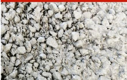
**BUNDREX 65/35CH** steel fibers are high quality structural steel fibers designed for reinforcement in shotcrete spraying. They are used successfully to replace the electro welded mesh in the reinforcement of tunnels, with an excellent performance proven with laboratory tests according to EN14651 and ASTM1609 standards.
