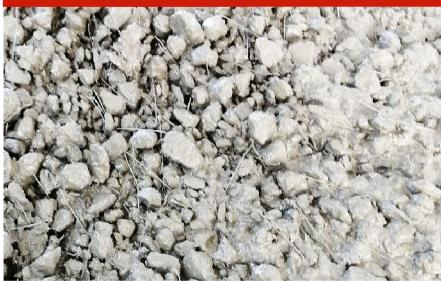
**BUNDREX 67/60CH** steel fibers are high quality structural steel fibers designed for reinforcement in Slab On Grade. They are used successfully to replace the electro welded mesh in the reinforcement of industrial floors with an excellent performance proven with laboratory tests according to EN14651 and ASTM1609 standards.
