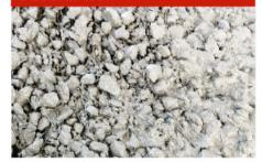
BUNDREX 50/30CH steel fibers are high quality structural steel fibers designed for reinforcement in shotcrete spraying. They are used successfully to replace the electro welded mesh in the reinforcement of tunnels, with an excellent performance proven with laboratory tests according to EN14651 and ASTM1609 standards.
