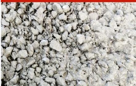
**BUNDREX 71/50CH** steel fibers are high quality structural steel fibers designed for reinforcement in Slab On Grade. They are used successfully to replace the electro welded mesh in the reinforcement of industrial floors with an excellent performance proven with laboratory tests according to EN14651 and ASTM1609 standards.
