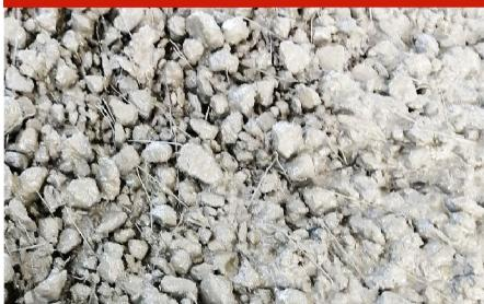
**BUNDREX 60/60CH** steel fibers are high quality structural steel fibers designed for reinforcement in Slab On Grade. They are used successfully to replace the electro welded mesh in the reinforcement of industrial floors with an excellent performance proven with laboratory tests according to EN14651 and ASTM1609 standards.
