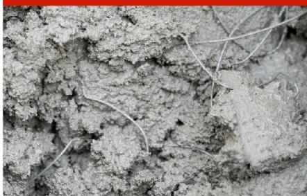
**SUPER BUNDREX 80/60CA** steel fibers are high quality structural steel fibers designed for reinforcement in Slab on Grade. They are used successfully to replace the electro welded mesh in the reinforcement of industrial floors, with an excellent performance proven with laboratory tests according to EN14651 and ASTM1609 standards.
